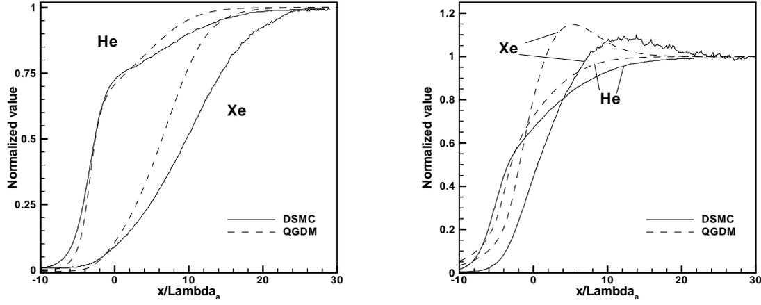
FIGURE 1. Density and temperature profiles in a He-Xe mixture
