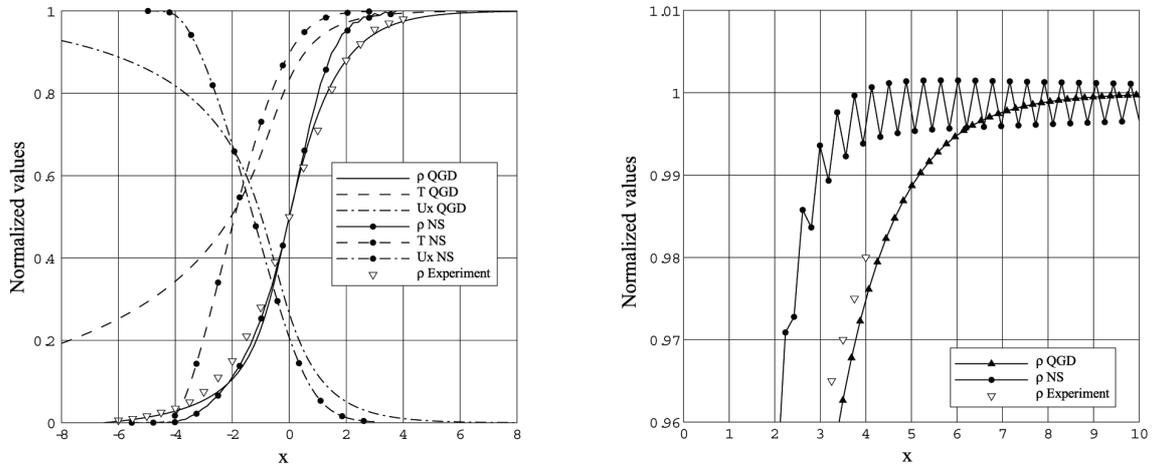
**FIGURE 1.** Density, velocity and temperature distributions in argon shock-wave,  $Ma=9$  (left). Fragment for the density distribution (right) Comparison of the QGD and NS solutions with the experiment.
