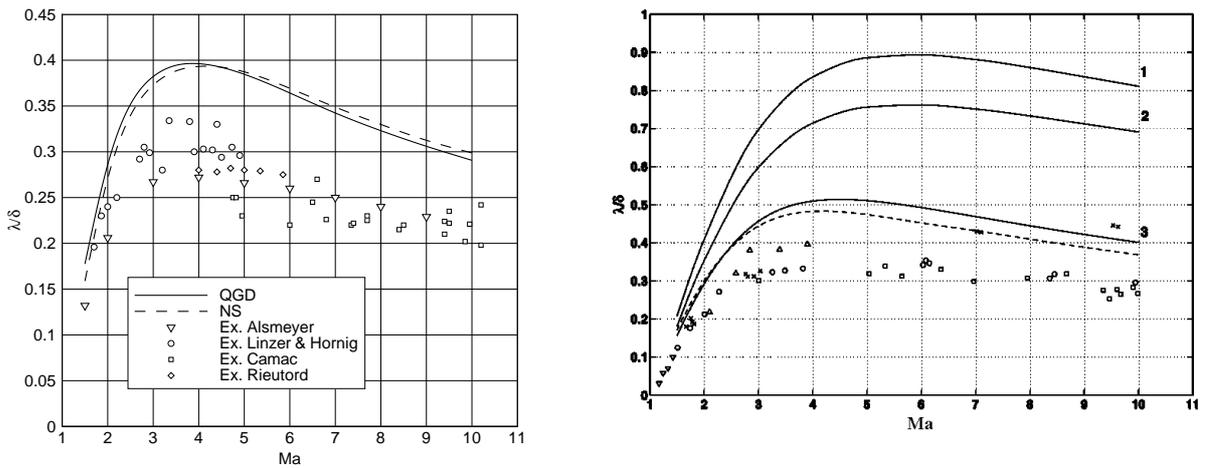
**FIGURE 2.** Reciprocal shock-wave thickness in argon (left) and nitrogen (right) compared with the experiment. Navier-Stokes computations - solid lines, QGD computations - dashed lines.
