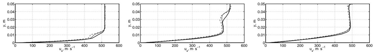
**FIGURE 3.** Longitudinal velocity profiles for the flow around flat plate at a distance from leading edge  $x = 4$  cm,  $7$  cm and  $10$  cm respectively, from left to right. DSMC calculations - solid line, QGD - bold solid line, NS - dashed lines.
